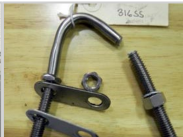
Figure 2 Bow Eye Tensile
