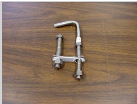
Figure 2 Bow Eye Tensile Failure
