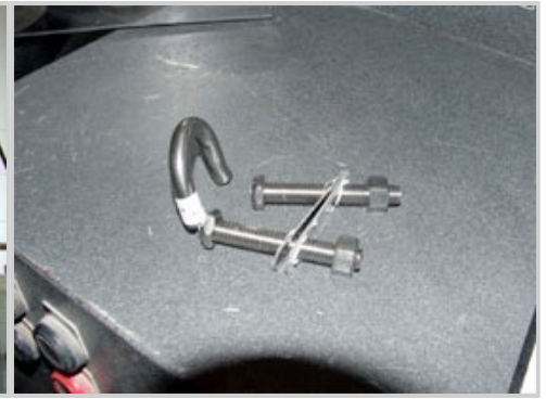
Figure 6 Side Pull Failure
