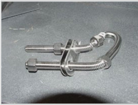
Figure 4 Bow Eye Edge Failure
